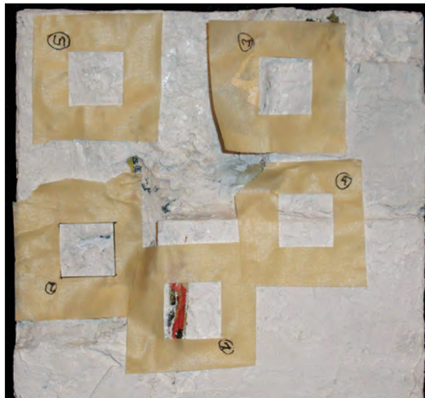
Fig. 3. The 5 areas of the same painting, shown in Fig. 2, with the 5 areas masked off that were scanned using Fourier-domain Optical Coherence Tomography. Photograph by Yao Xiao © Yao Xiao, 2012. Used with permission.
